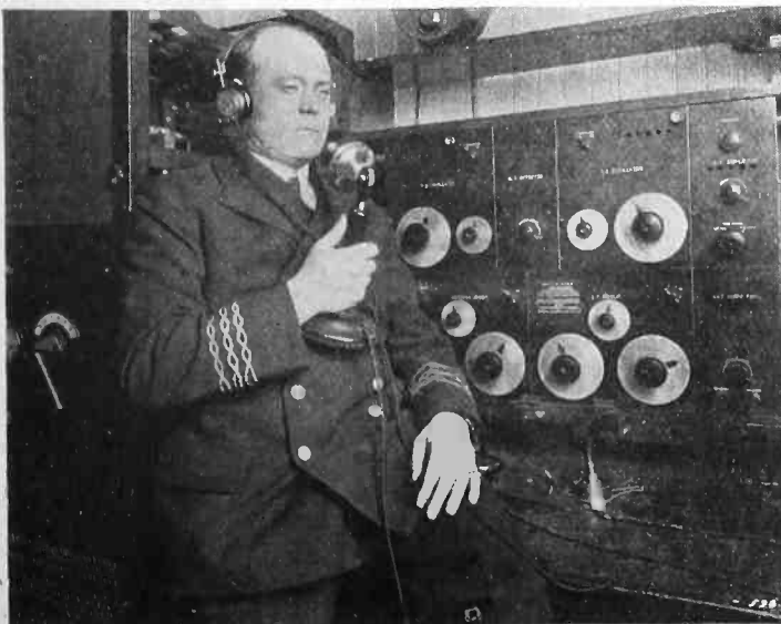
Chief Radio Officer aboard the S.S. Leviathan speaking over radio telephone (Duplex System) installed by Radio Corporation of America.
